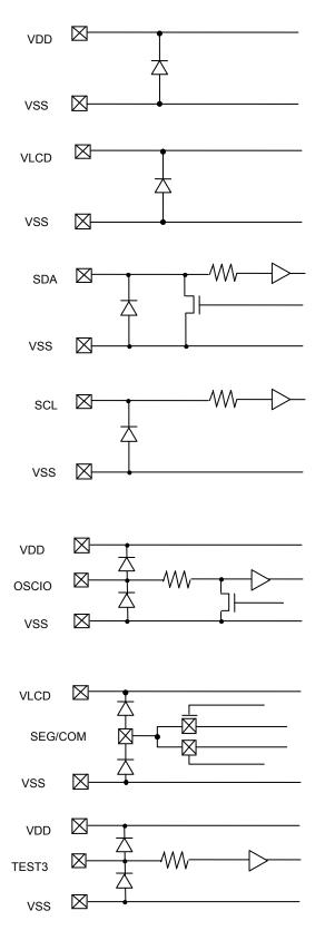
Fig. BU9799KV-7 I/O equivalent circuit
