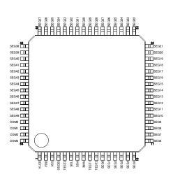
Fig. BU9799KV-3 Pin arrangement
