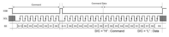
Fig. BU9794KV-4 3-SPI Command/Data Transfer format
