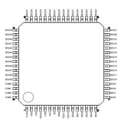
Fig. BU9794KV-3 Pin arrangement
