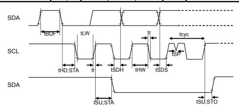
Fig. BU9799KV-1 interface timing
